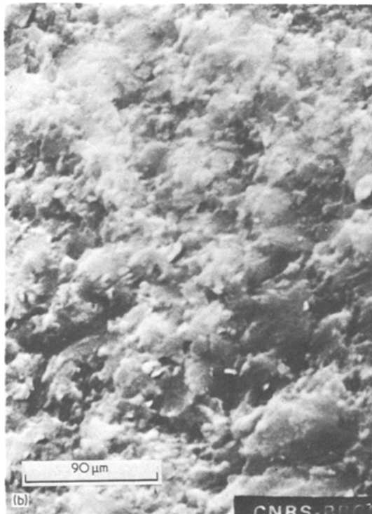
Figure 15 Microstructure of (a) hardened cement paste in unimpregnated concrete, (b) impregnated hardened cement paste.
